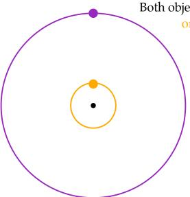
Both objects are moving at a rate of 30 rpm. The radius of the orange circle is 3 ft and the radius of the purple circle is 12 ft. What is the linear speed of both objects.
