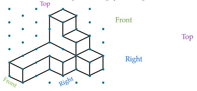
Convert the isometric drawing into a foundation drawing
