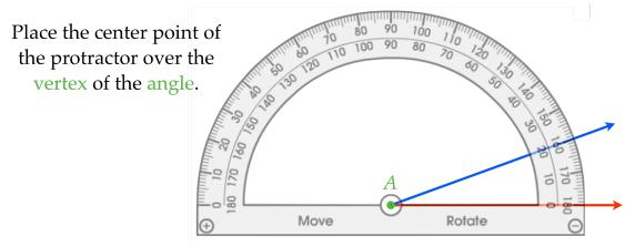
Align one side of the angle with the 0° mark of the protractor
