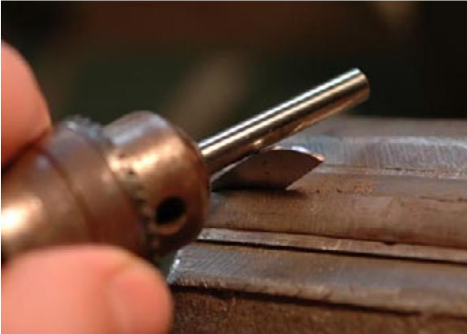
I beveled the curved edge so that I could get the blade right up to the perpendicular section that I was carving. Wood scrapers are sharpened by rolling a burr up on the edge. A good tool for this is a worn out carbide end mill. They are common in my shop, but you can pick one up from a local ma-
