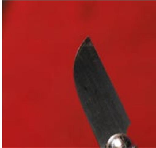
With a micro burr on the edge you can pull dust off the carving with little effort. The finished scraper is ready to use in a useful and inexpensive handle. You can make the blade to any shape with a grinder or file and fit them to the handle quickly. Notice the fine burr on the curve.
