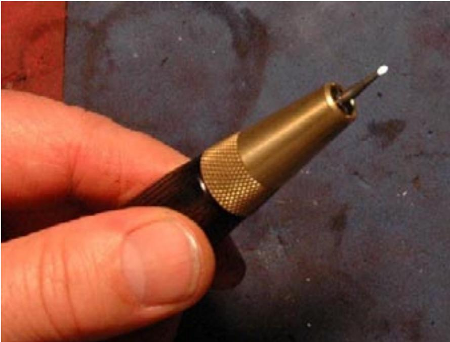
**Dental burr cutter** - Break off the end of a used dental burr and then grind and shape the tip to suit. The chuck holds it solidly and the handle is great.
