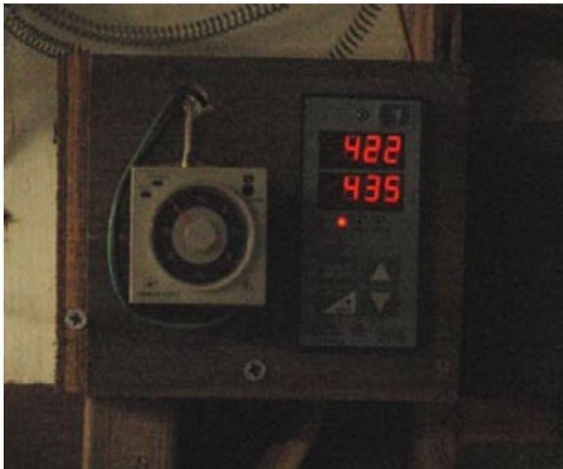
**Tempering** - Heat in oven at 425 degrees F for one hour.
