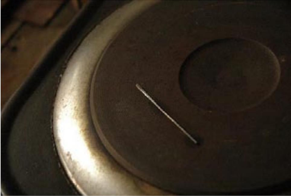
**Step5: Tempering** - Sand off the chisel to bright metal and place on a hot plate. Turn to medium high and watch the colors on the bright section. Take off the hot plate when the color gets to bronze. Let cool.
