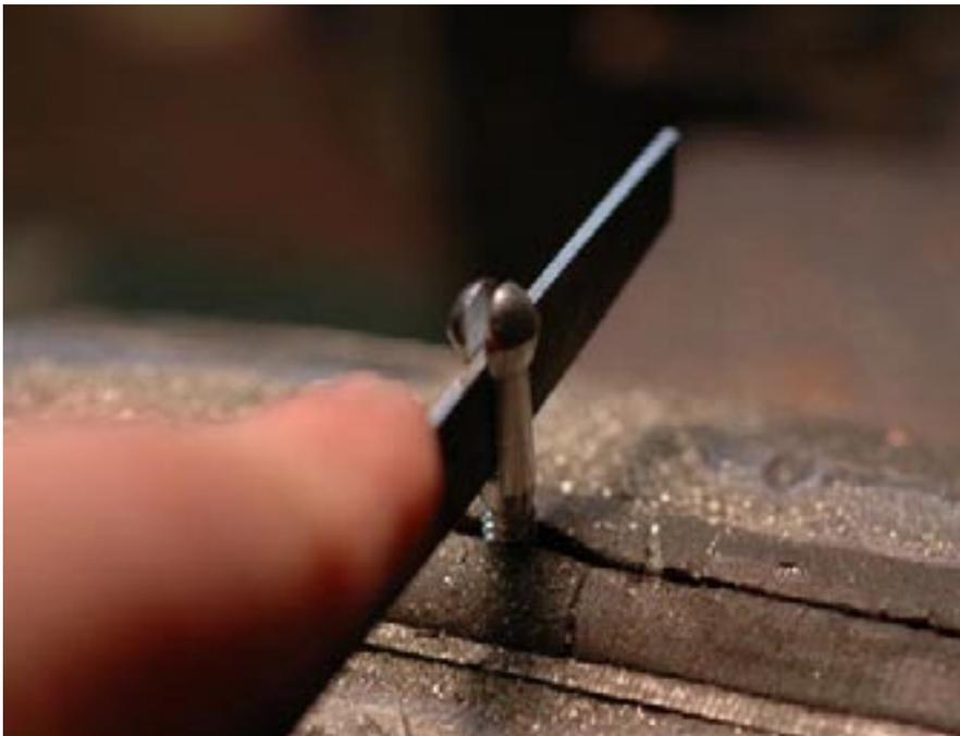
**Filing collet** - Depending on the size stock you use for the blades you may have to widen the collet by filing to accommodate the thickness
