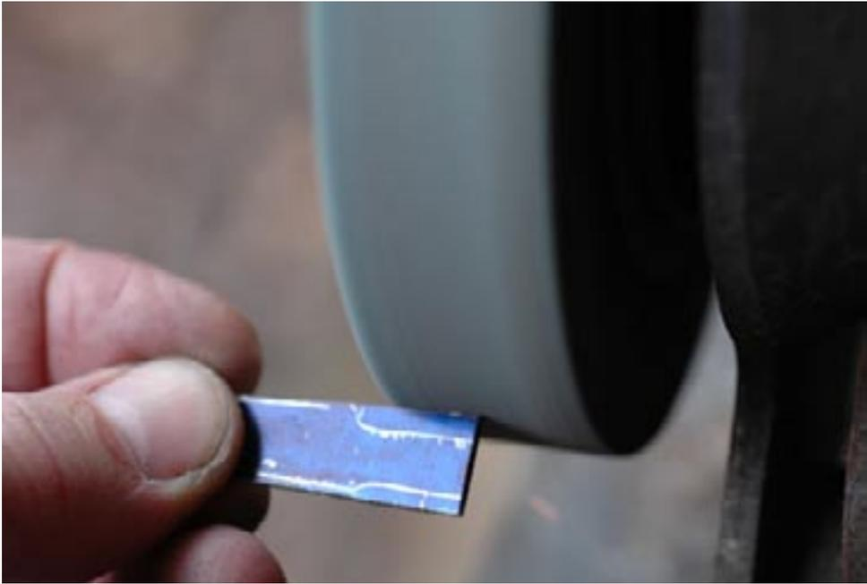
The blade is shaped using a simple rock grinder. I had to tie up one hand with the camera, but you get the idea.
