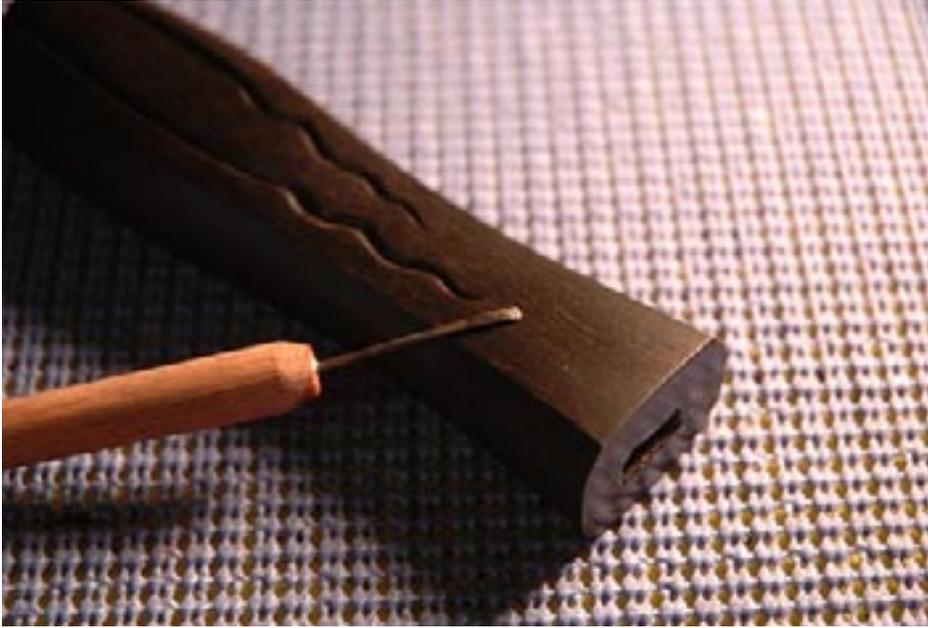
**Step 7: Mount in dowel for handle** - Mount in a piece of dowel and sharpen. You can quickly make specialized chisels and knives for micro carving.
