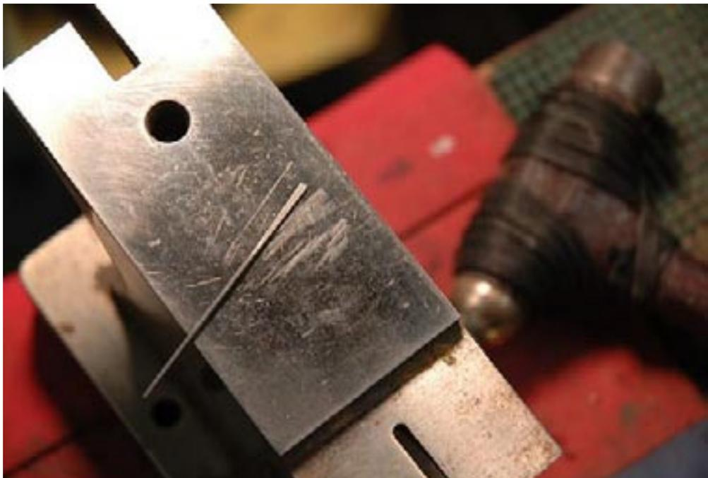
**Step 2: Cold work** - Flatten the wire cold. You can form it over a round to induce slight curve.
