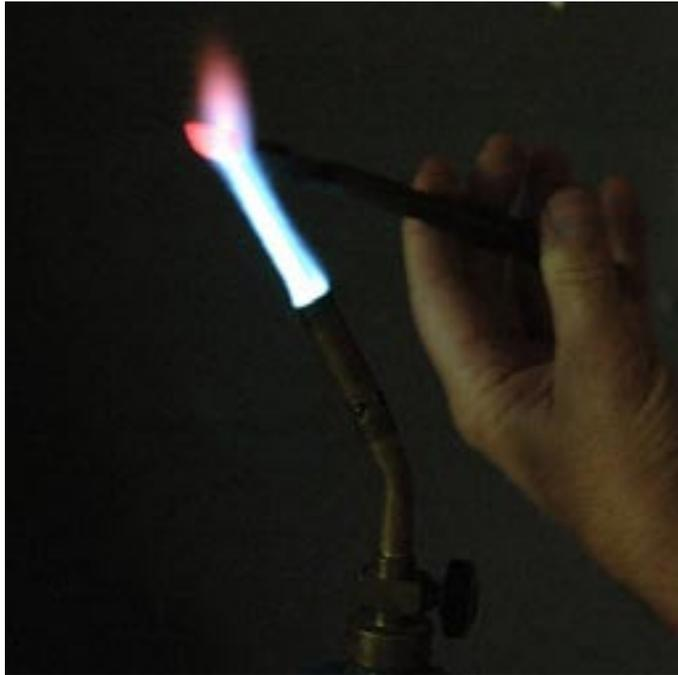
**Hardening blade** - Using a plumbers torch heat the blade to an even orange heat and then quickly plunge into canola oil
