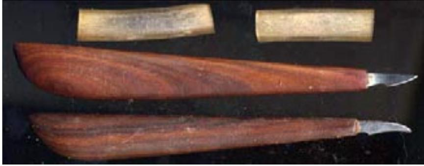
Here are some pictures of the tools. The little chisels with the octagonal handles are commercially available Dockyard brand, and I like them a lot. The round handled ones are just flats made by me from piano wire available at hobby shops with the balsa wood. The light colored handle is a shaker peg available a woodworking stores and a nice quick and dirty handle solution. The clear plastic tubing in the pictures is used to cover the business ends of chisels and knives for safety.
