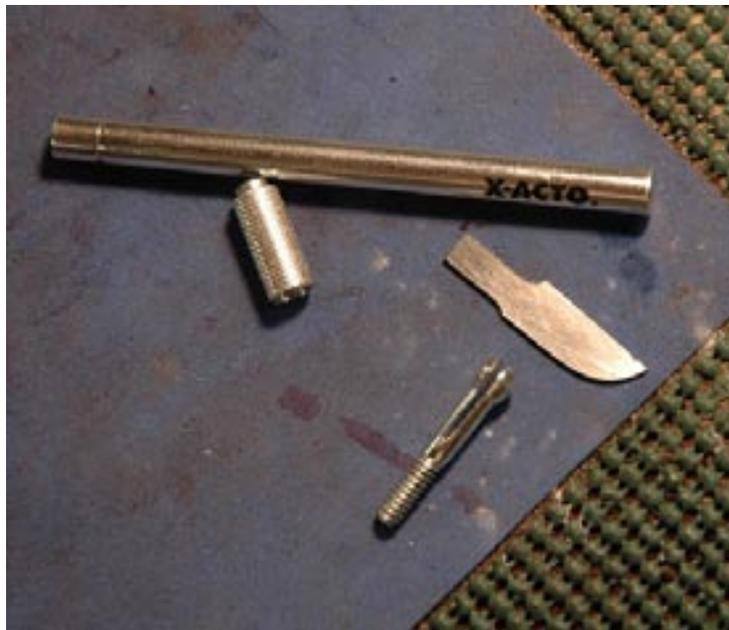
The screw is the base of the collet for this knife. Xacto makes it and they sell for around \$2. I just widened the collet so it would take the slightly large stock I am making the blades from.
