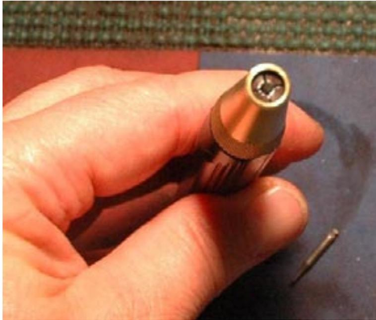
**Veritas chuck** - To use with dental burs loosen the chuck so that it spreads to maximum opening and then drill out the center with a 5/64ths drill. It will chatter some.
