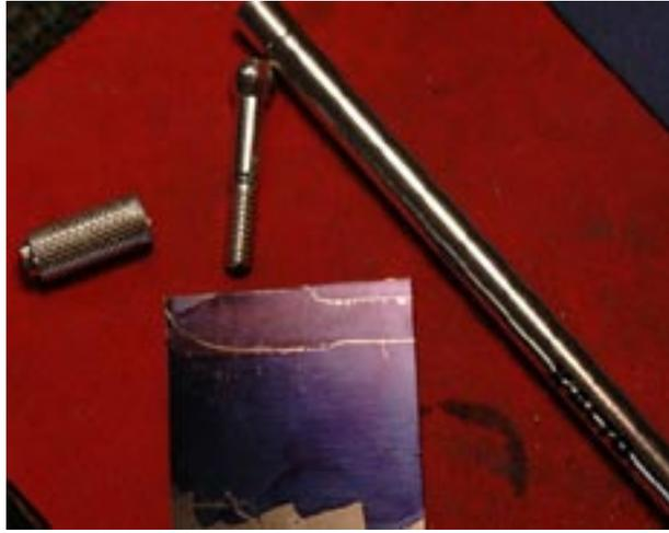
I am discovering that tool making is a large part of doing carving. One of the tools that I found myself making were scrapers. What I did was adapt a cheap Exacto handle to accept a thicker shaped scraper.
