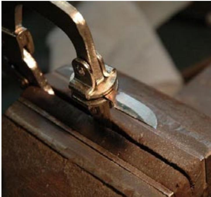
**Filing blade** - Cut out the blade profile with a saw and hard wheel grinder. The bevels can be filed in.
