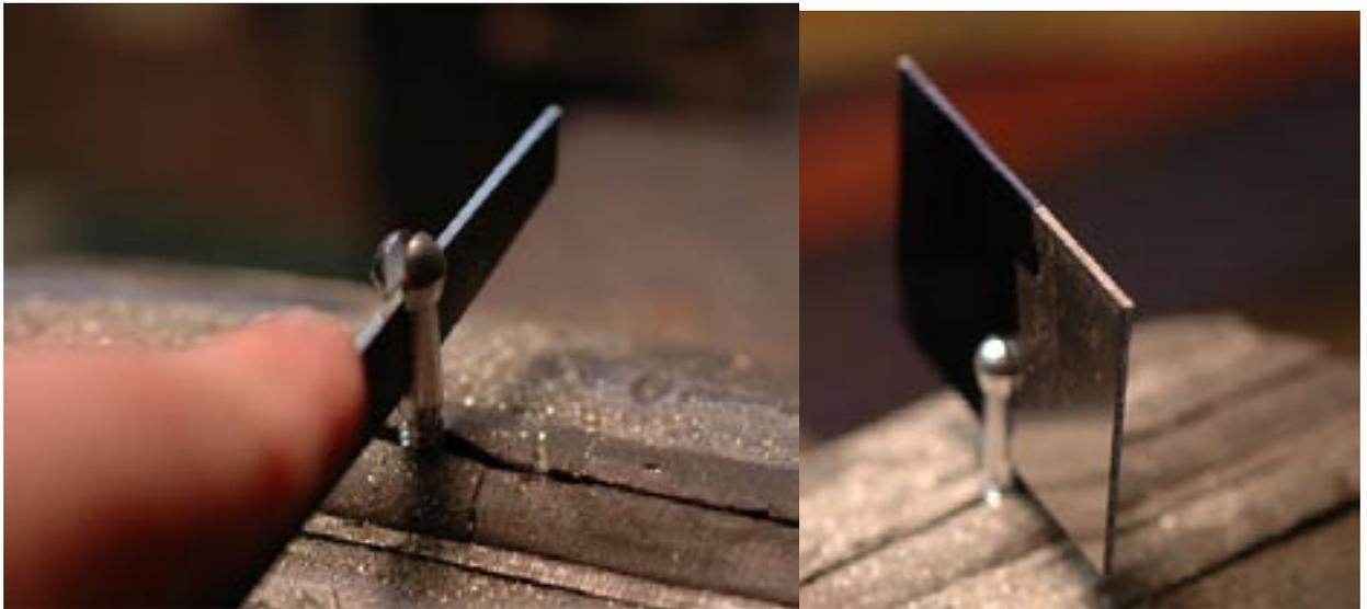
For the steel, I used 3/32nds 15N20 tool steel. This is a high nickel content steel that even unhardened has good toughness. It can be bought in small quantities from Swain Spring Shop, Jeff Carlisle, 1-406-452-1246.
