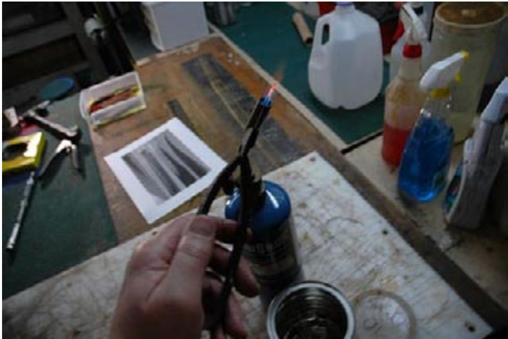
Step 4: Hardening - Heat with a propane torch to a nice even color and quench quickly into mineral oil. Check with a file, if it has hardened the file will skate without biting. If it didn't harden reheat and get it a little hotter and re-quench.
