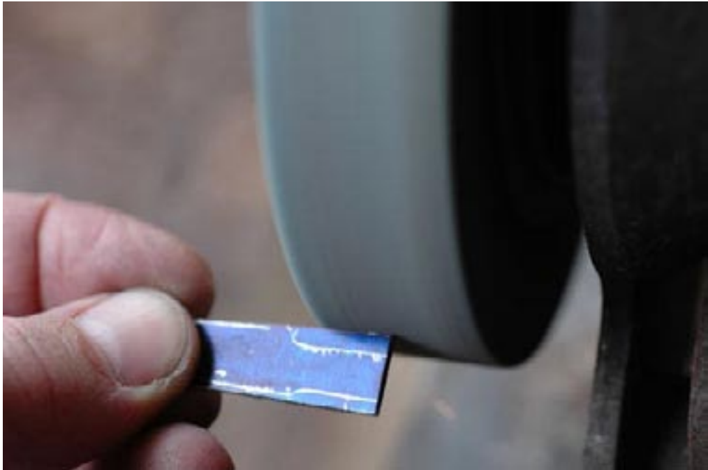
Grinding blade - Profile the blade with a hard wheel grinder
