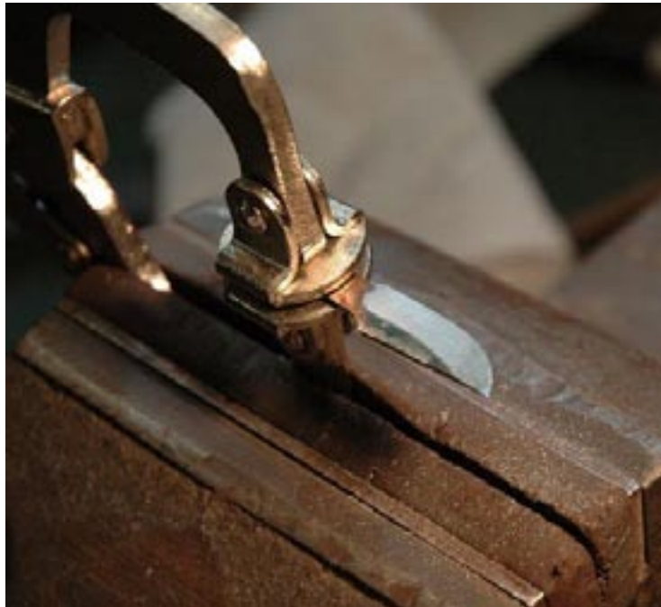
Filing blade - Cut out the blade profile with a saw and hard wheel grinder. The bevels can be filed in.
