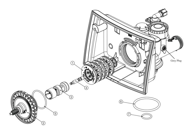
XT-32C Drive Cap Assembly, Downflow Piston, Regenerant Piston and Spacer Stack Assembly
