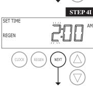
STEP 4I – Next Regeneration Time (hour): Set the hour of day for regeneration using ▼ or ▲ buttons. AM/PM toggles after 12. The default time is 2:00 a.m. Press REGEN to return to previous step.
