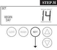
STEP 3I – Days Between Regeneration (Days Overide): The manufacturer has factory set 14 days as the default. This is the maximum number of days between regenerations. If this is set to "OFF" regeneration initiation is based on gallons used only. If any number is set (available range is from 1 to 28 days), regeneration will be called for on that day even if a sufficient number of gallons were still available. Set Day Override by using the ▲ or ▼ buttons.
