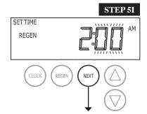
RETURN TO NORMAL MODE **STEP 5I** – Next Regeneration Time (minutes): Set the minutes of day for regeneration using  $\nabla$  or  $\triangle$  buttons. Press NEXT to exit Installer Display Settings. Press REGEN to return to previous step.
