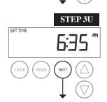
STEP 3U - Current Time (minutes): Set the minutes of the day using ▼ or ▲ buttons. Press NEXT to exit Set Clock. Press REGEN to return to previous step.
