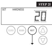
STEP 2I – Hardness: Set the amount of hardness in grains of hardness as calcium carbonate per gallon using the ▼ or ▲ buttons. The default is 20 with value ranges from 1 to 150 in 1 grain increments. Note: The grains per gallon can be increased if soluble iron needs to be reduced. This display will show "–nA–" the system is set up for a filter or if 'AUTO' is not selected. Press NEXT to go to step 3I. Press REGEN to exit Installer Display Settings.
