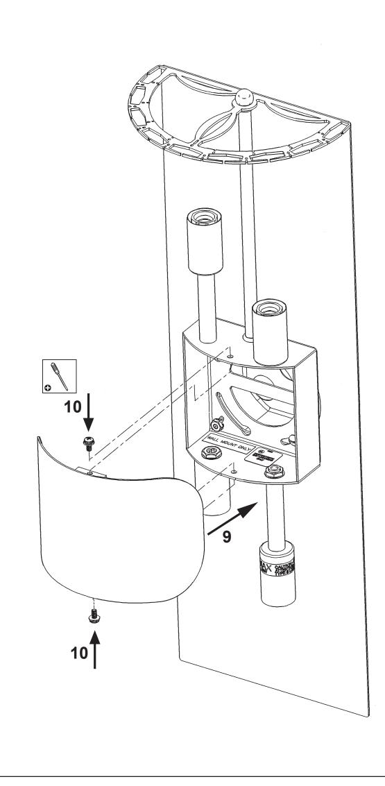
You will need 4 - B10 25 Watts Recommended 60 Watts Max Install bulbs and be sure to test fixture BEFORE trimming.
