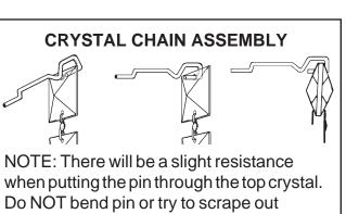
when putting the pin through the top crystal. Do NOT bend pin or try to scrape out crystal hole. The resistance holds the crystal chain on the pin.
