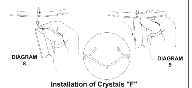
Hook Crystal "F" into the curve of the "scalloped" ring. Hold hook with index finger and thumb. Slide hook from behind scalloped ring. (Diagram 8)
