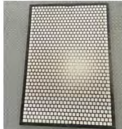
Screens: Pre-tensioned shaker screen
