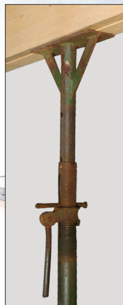
Long post-shore jacks are useful for several of these suggested stiffening strategies. They vary in price, depending on lifting capacity; prices start around $25 apiece ( www.ablebuilders.com ).
