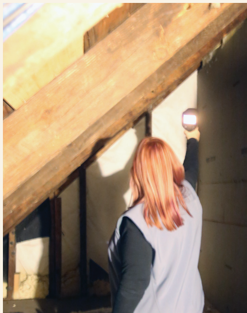
Infrared insights. With the infrared camera, we scan the exterior walls, particularly where they meet the floors and ceiling, and we verify issues, like leaky and uninsulated kneewall attics and attic hatches.
