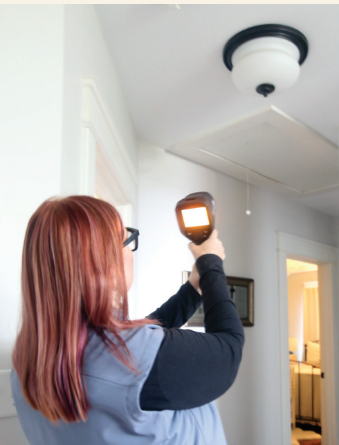
Infrared insights. With the infrared camera, we scan the exterior walls, particularly where they meet the floors and ceiling, and we verify issues, like leaky and uninsulated kneewall attics and attic hatches.
