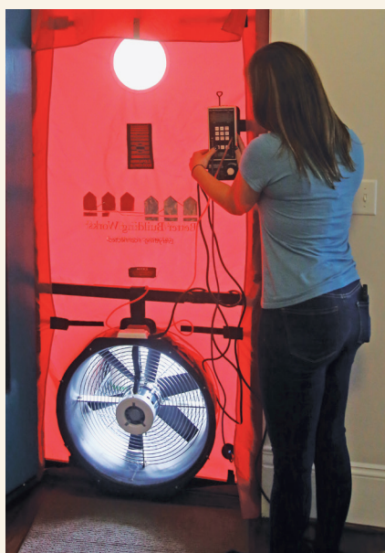
Blower-door benefits. Blower-door testing reveals more than just how tight or leaky a house is. By running the fan while we look around with the thermal camera, we can often locate the leaks. Follow-up tests after upgrades are complete allow us to verify that the work was successful and to accurately size and commission HVAC equipment.
