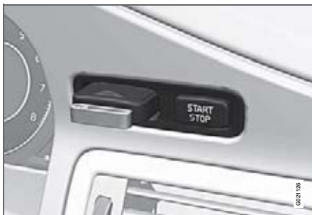
Ignition switch with remote control key, start and stop button (see more information on page 65).
