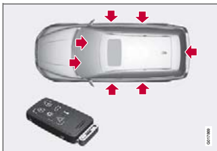
Active locks for remote control key, with key blade and privacy locking not activated.
