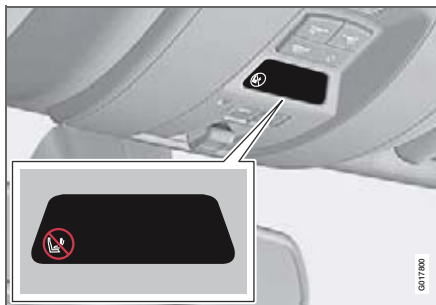
Indicator in roof console showing that the passenger airbag (SRS) is activated.
