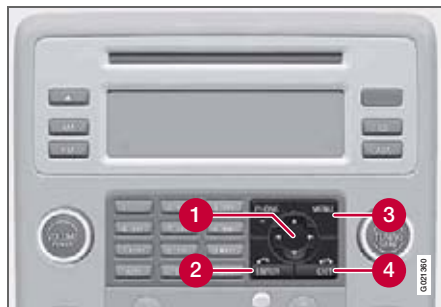
Centre console with information display and controls for menus.
