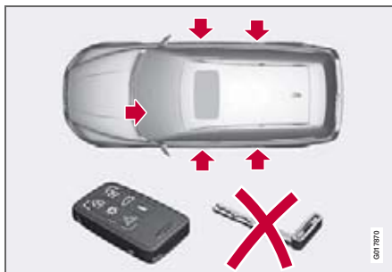
Active locks for remote control key, without key blade and with privacy locking activated.
