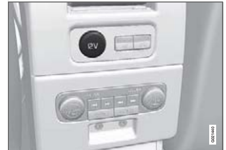
12 V socket in tunnel console, rear seat.
