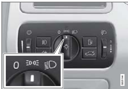
Headlamp control in position for position/parking lamps
