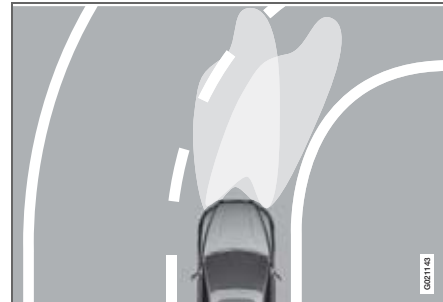
Headlamp pattern with function deactivated (left) and activated (right) respectively
