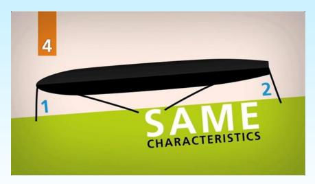
Mooring lines 1 and 2 should have same specifications: length, elasticity and tension
