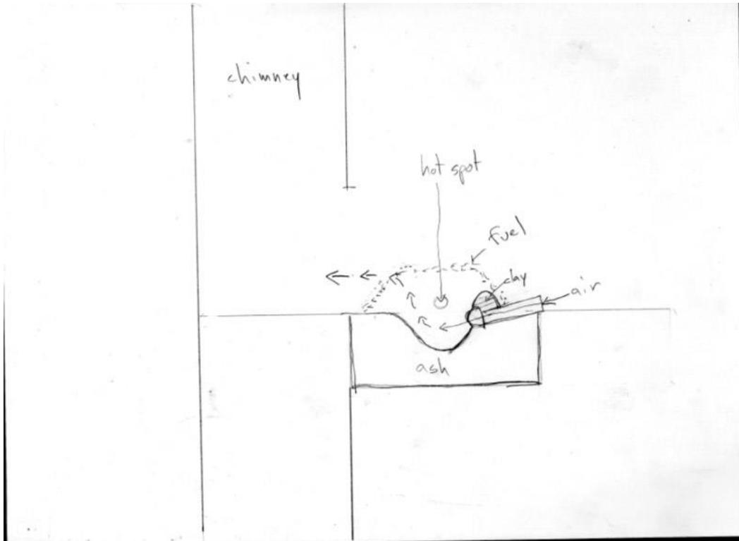
I generally have to reshape the duck's nest every month or so with fresh wood ashes. The advantages of using the wood ashes are both the ability to reshape the duck's nest as necessary, and its insulative qualities.
