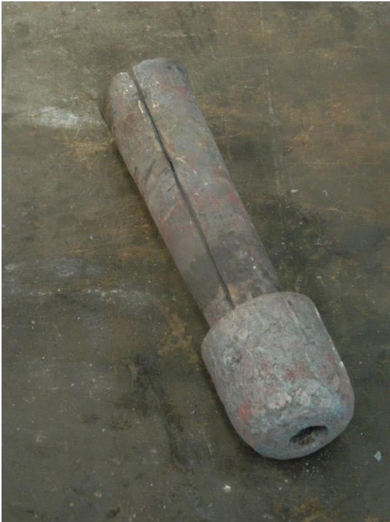
A wise person would immediately make another one, so you when it fails or you need to reforge it, you have a good one to install. Over time, you will find the top will erode, and the orifice will enlarge, as seen in the original. Then you can just reforge it back to the proper shape
