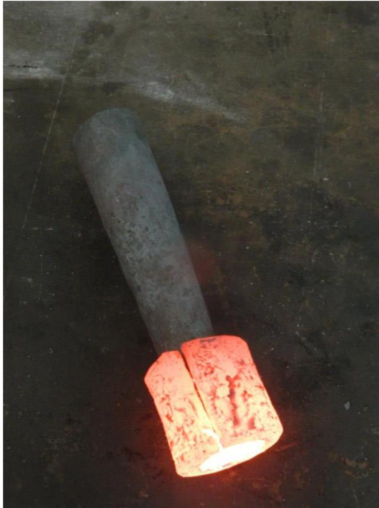
Then flux it, and weld it all up in the swage block. Take your time and take a nice slow heat, so the inner tube has time to get to welding heat. Don't forget you can look down the tube to see if it's really hot, just looking at the outside can fool you!
