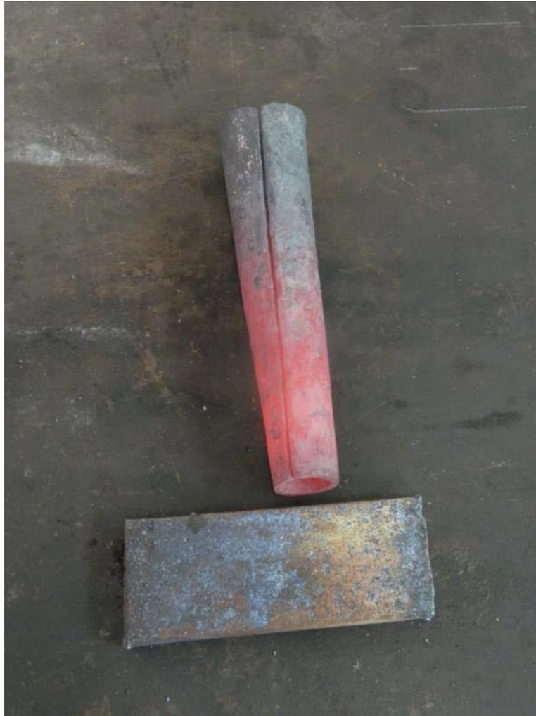
Then wrap the 5/8" x 3" stock into a collar, and drive the tube into it. You want to leave a bit of gap on the collar, say a 1/4". It's nice to have the tube extending at least halfway into the collar, for lots of welding surface:
