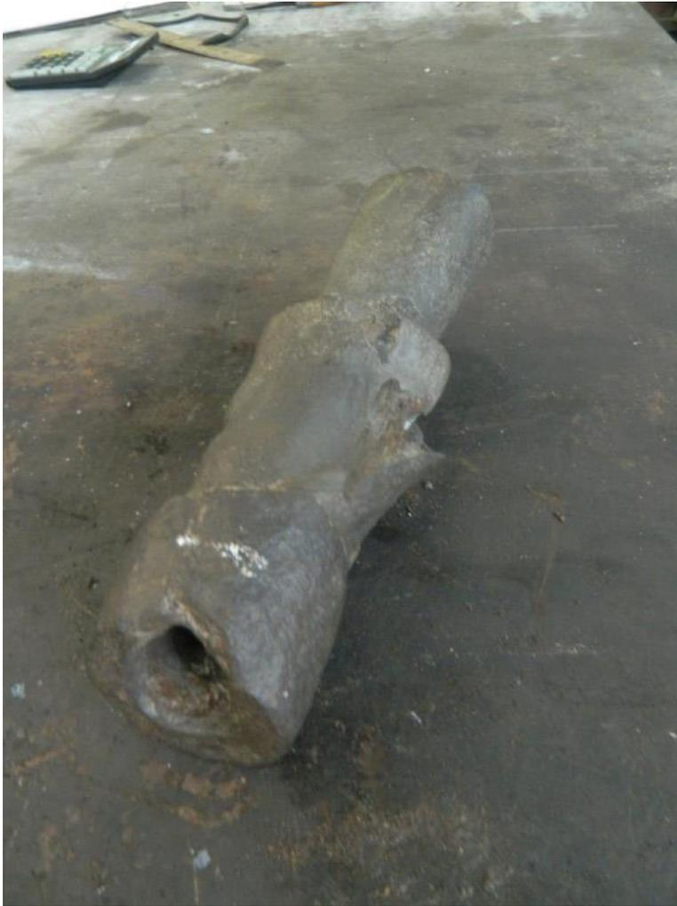
I had already tried a wrought iron tube as a tuyere, and despite wrought's high melting temperature, it had burned out almost immediately. We were intrigued by this design- by building up the end of the tube by forge welding, perhaps we'd get something more durable.
