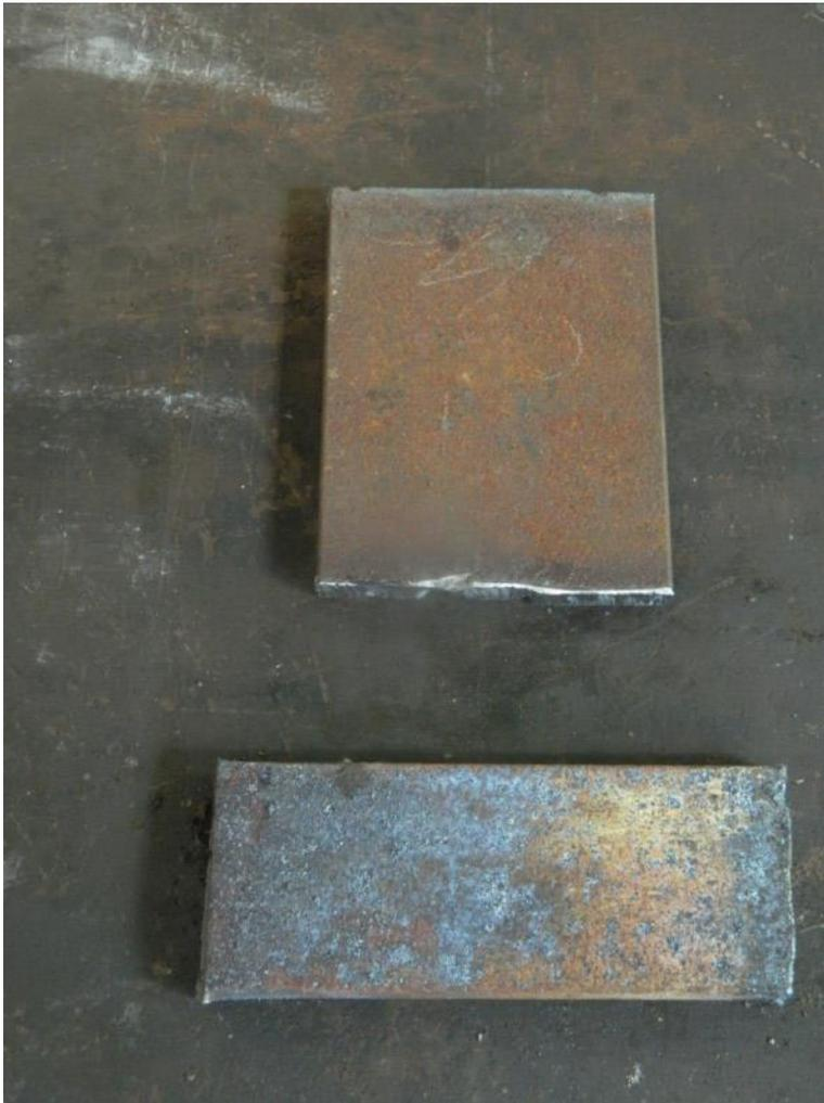
Then I forged the  $\frac{1}{2}$ " x 5" into a trapezoidal plate, roughly  $\frac{1}{4}$ " thick. The finished trapezoid is 5" wide on the narrow end, 7" on the wide end, and  $10\frac{1}{2}$ " long. If you have a nice piece of  $\frac{1}{4}$ " wrought plate, of course you'd just cut this out of that! The length is not critical as it is with the copper tuyere, this is just a convenient length for my set up.
