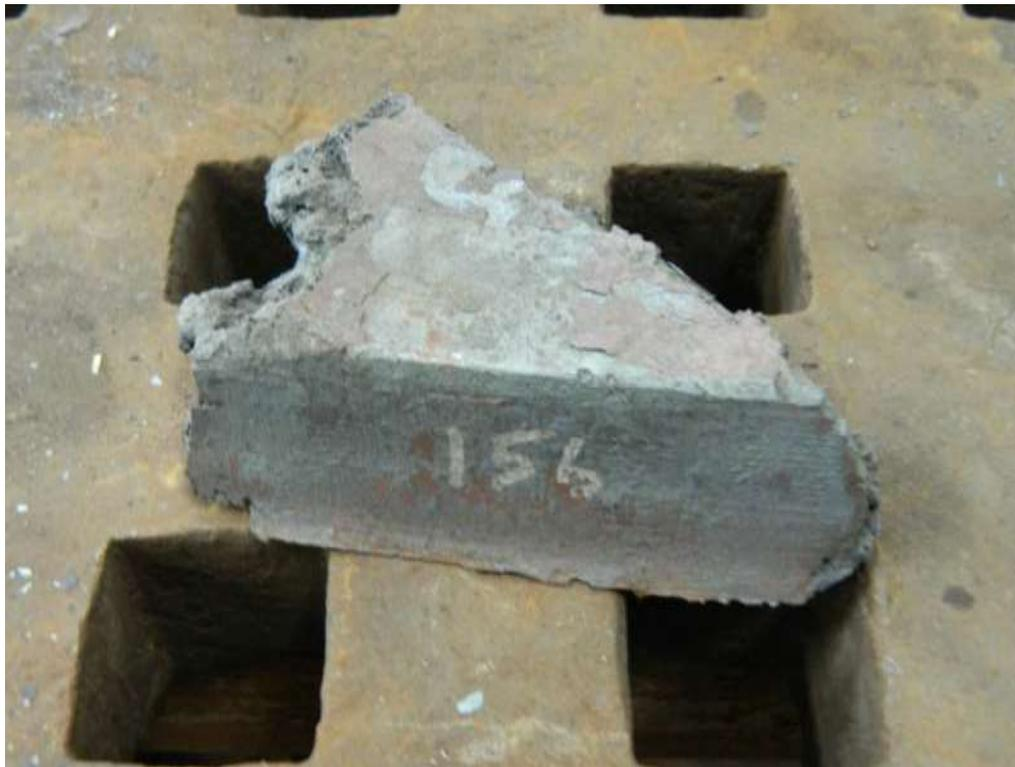
Then I remelted a quarter bloom from smelt #156, weighing 4.4 lbs, in a hearth with the tuyere 1¼" above the hearth floor. After remelting and (and slightly flattening) the resulting bloom weighed 2.5 lbs. I scored the bottom of this remelted bloom, and folded it, thus welding it face to face, and drew it to a ¾' x 2" x 5" bar that weighed 1.83 lbs. I sliced a cross section of this bar for a metallographic sample at this point.
