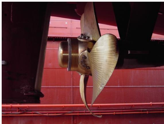
**Figure 4.3 Kappel Propeller**
