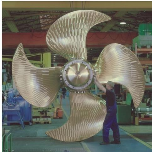
**Figure 4.1 Highly skewed propeller**
