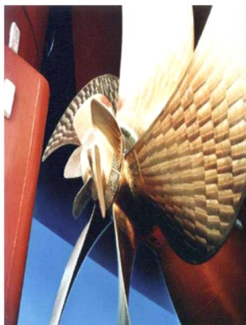
**Figure 5.1 Propeller Boss Cap Fins
