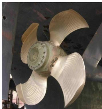
**Figure 4.2 Typical CLT propeller**
