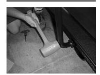
Use a soft mallet to firmly set the rails inside the clamp.
