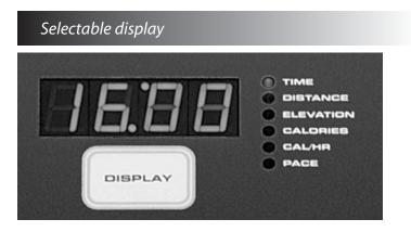
The **DISPLAY** button allows you to move about the selectable display. You can move the selectable display automatically from option to option by using the Scan mode. Press and hold the **DISPLAY** button for 3 seconds to enter the Scan mode. When in the Scan mode the display will advance by itself every five seconds. Press the **DISPLAY** button one more time to exit the Scan mode.
