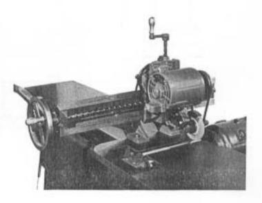
In the picture above, the bar is located occurately by the two tapped holes. The cutterhead or cylinder is located by the dowel pin. The mater bracket is clamped to the slide block by a hand knob, and the slide block is actuated by the crank shown at the left end. The cylinder remains stationary while the grinding wheel is fed taking a light cut. The next knife is brought in place by pulling out the dowel pin and rotating the cylinder by hand.
