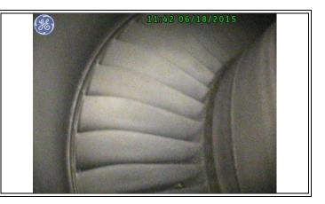
Combustion Liner, No defects noted
