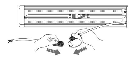
Remove the cap and align the arrows
