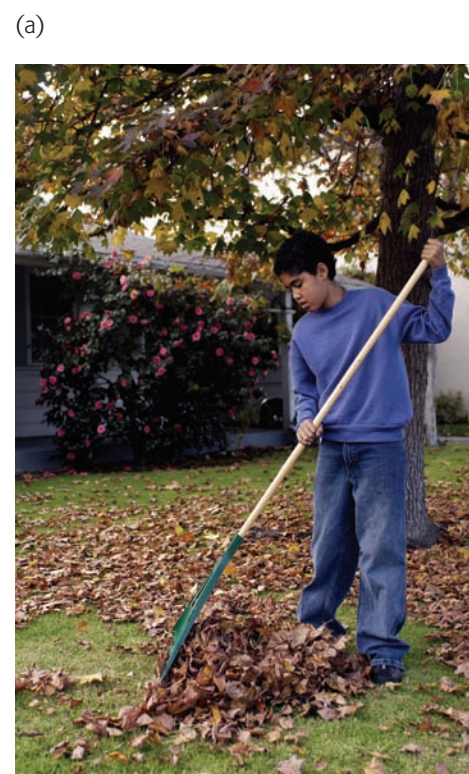
Figure 5.9 A garden rake is an example of a third-class lever, which has the input force between the fulcrum and the output force.
