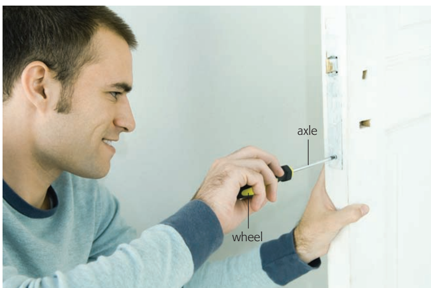
Figure 5.20 (a) A wheel and axle. (b) A screwdriver is an example of a wheel and axle.
