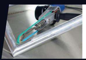
Belt File BFS650 for edges, corners and grooves. Ideal for high stock removal application in hard to reach areas as well as surface preparation and finishing. Allows a penetration up to 200 mm with a 650 mm belt length. Accomodates belt widths of 5 and 12 mm. Safe belt guidance even when used with 5 mm belts.
