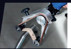
**Pipe Belt Sander** PBS650/760 for grinding, finishing and polishing tubes up to 6" in diameter. Belt sizes  $15/35/40 \times 650$  mm. Optional belt size  $15/35/40 \times 760$  mm with a longer pivot arm. Up to 9" in diameter.
