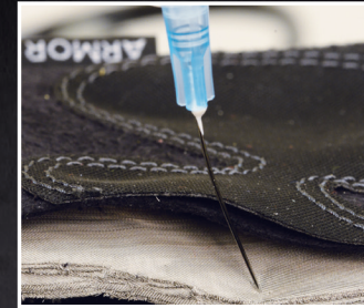
25 gauge needle buckling
