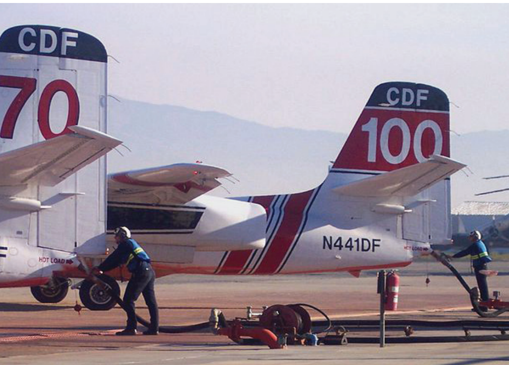
Tanker 70 and 100 reloading at Hemet-Ryan Airport, California. Photo: Lvi56
