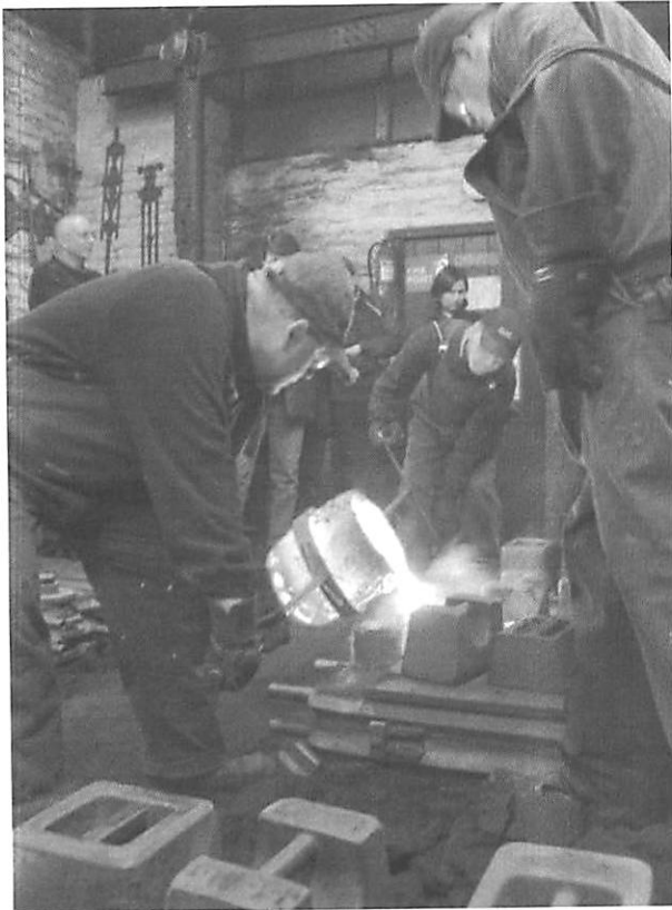
Figure 3. Casting grey iron into green sand molds at Beaverbank Foundry, Edinburgh, in 2004 (Copyright, D.S. Mitchell)
