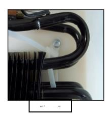
**4.** Verify the tabs on the RC evaporator cover are not broken or missing screws, and the insulation on the inside of the cover is not damaged or making poor contact. If any tabs are broken (See Figure 8) or the insulation is making poor contact replace the cover per your model's RPL. Replacement screws are available (part# 67006425).
