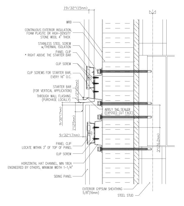
THROUGH WALL FLASHING (Hat Channel/Vertical)
