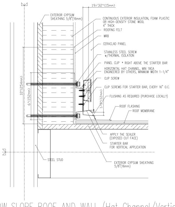
LOW SLOPE ROOF AND WALL (Hat Channel/Vertical)
