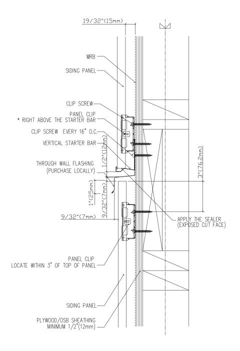
THROUGH WALL FLASHING (Wood/Vertical)
