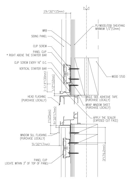
WINDOW AND DOOR HEAD AND SILL (Wood/Vertical)
