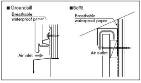
FIGURE 1—PANEL INSTALLATION
