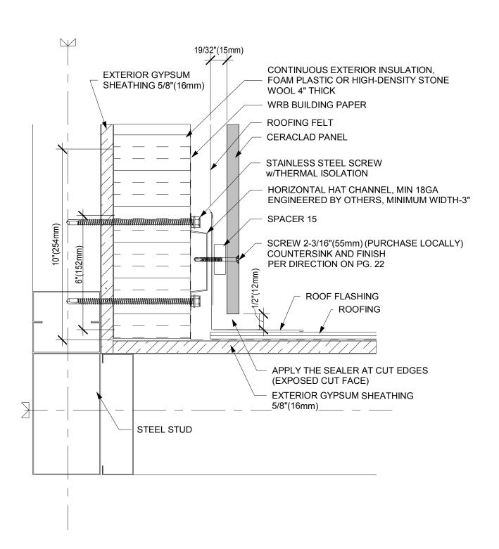
LOW SLOPE ROOF AND WALL (STEEL STUD) CERACLAD SIDING PANEL (16mm)
