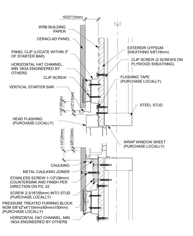
THROUGH WALL FLASHING (STEEL STUD)
