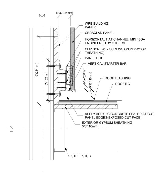
LOW SLOPE ROOF AND WALL (STEEL STUD)
