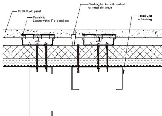
**When joints fall in between studs, metal strapping or flatstock can be added to span the studs. The minimum acceptable gauge for this flat stock is 18 gauge.**
