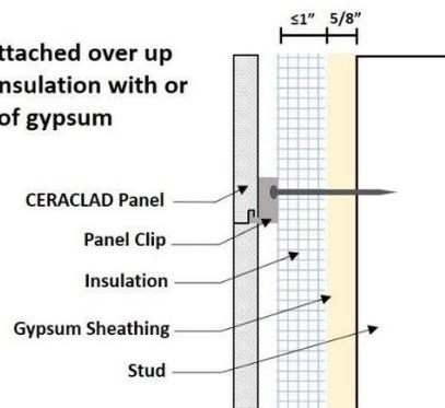
**For attaching CERACLAD directly through non-structural substrates, the following criteria must be followed:**
