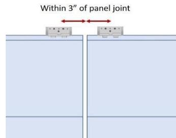
Clips shall be placed within 3" of each panel end. Additional blocking at joints may be required to accomplish this
