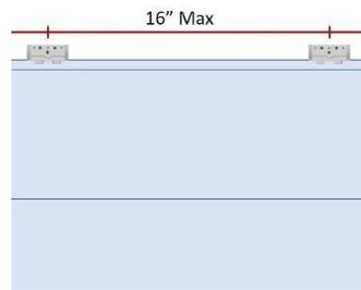
Panel clips shall be spaced 16" OC or less along the panel edge
