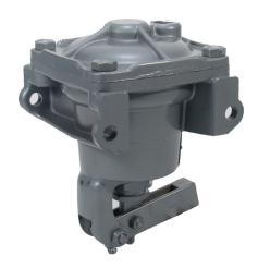
The A-2-H Actuator Positioner is a pneumatic positioner used where accuracy is required and when the device to be operated has low-force characteristics. Typical applications are positioning the butterfly valve of carburetors and the control arm of diesel engine governors.
