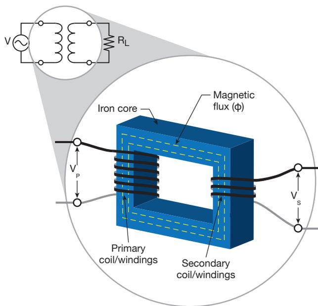
**Figure 1** This figure shows the symbol commonly used to represent a transformer in electrical diagrams (top left), as well as the components in a basic two-winding transformer (foreground). Since the voltage ratio is proportional to the winding turns ratio, the secondary voltage ( $V_s$ ) in this example equals one-half of the primary voltage ( $V_p$ ).
