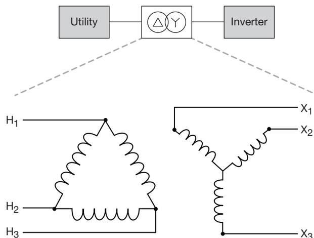
**Figure 3** The most common distribution transformer winding configuration in solar applications is the delta-to-wye with wye grounded or ungrounded.
