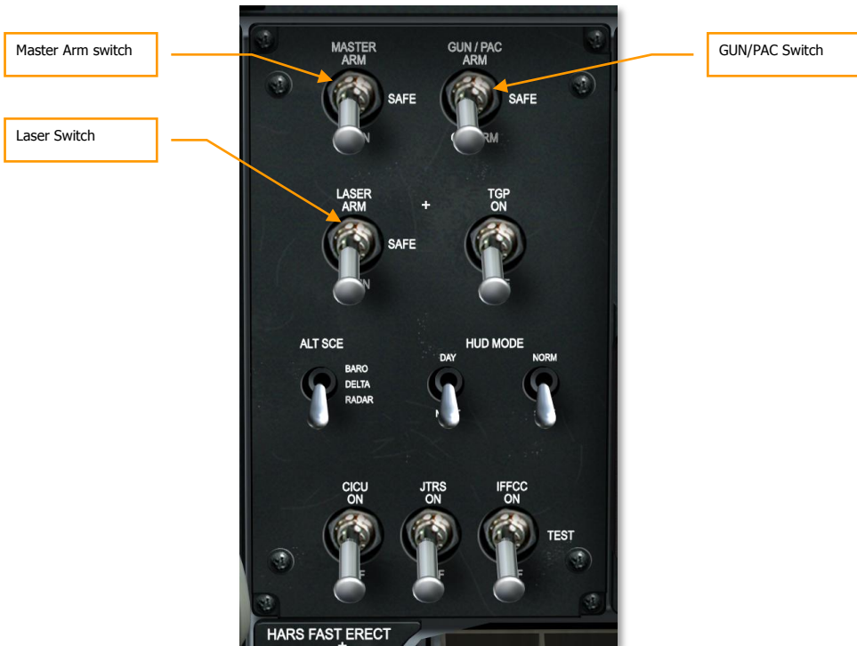
Figure 385. Armament HUD Control Panel
