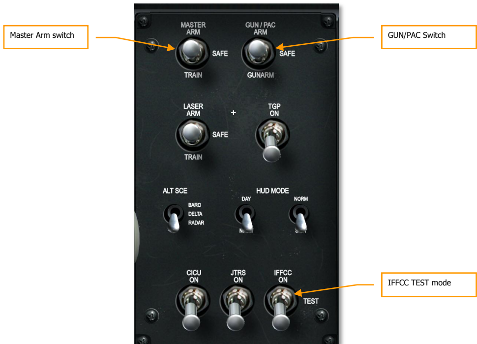
Figure 400. Armament HUD Control Panel
