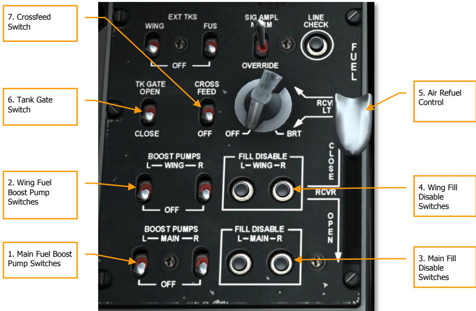
Figure 298. Fuel System Panel
