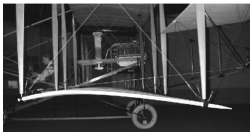
Figure 1. Curtis 1911 model D type IV pusher
