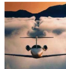
Figure 7. Downwash and wing vortices in the fog.
