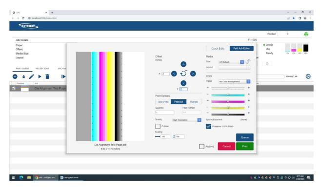
6. The job should be run with a 9x12 envelope with the flap side run against the fence on the alignment section. The cyan bars as shown in the image above should be printed on the leading edge of the envelope and offset horizontally by 2 inches. This offset should put the resulting print in the middle of the envelope. The color profile should always be No Color Management to avoid all four colors mixing together in each color bar. Print the job.
