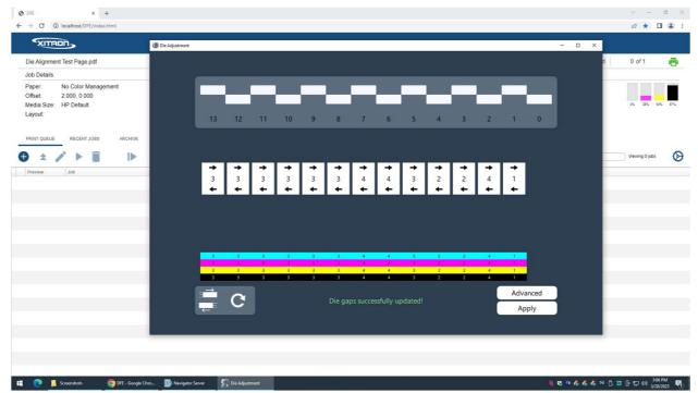
2. Moving from right to left, line 1 looks nice, so leave that for later. You may notice a line that looks like a gap in die 4. This is a normal streak that can appear often and is fixed by doing a mid-job service or a pen recovery. The most offensive lines are lines 2, 5, 6, and 7. To fix them, move dice 2, 5, 6, and 7 to the right as shown below:
