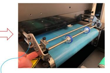
Hold the assembly up in the slots so that it is tightened at the highest position.
