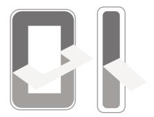
Step 3 - Clean the surface on which the door sensor is to be installed, align the sensors and glue them tightly on the door
