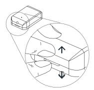
2 Pull out the used battery and replace with a new one
