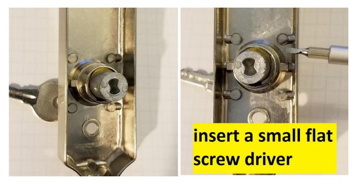
**Step 3:** Depress the brass color part, then push the key cylinder out.
