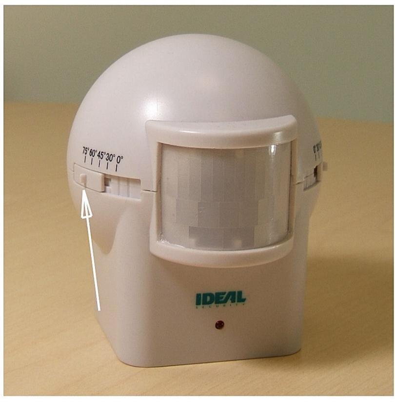
You can slide open the sliders to maximize the detection range. (zero detection at  $0^{\circ}$ , max detection at  $75^{\circ}$ )
