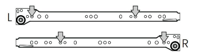
Use the hardware ( C ) to apply the slides 18 on the parts 16 and 17.
