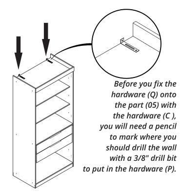
\*press the hardware wings (P) to put in the hole that you drilled in the wall.
