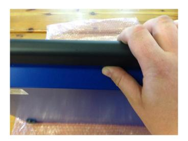
Gently open the console as shown. Note DO NOT open more than 45 degree's from the base as damage can be caused to the battery connector.
