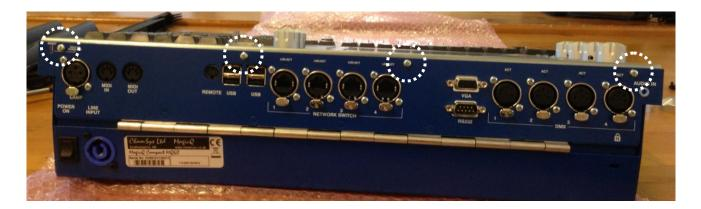
Turn the console around and remove the 4 of M3 x 5mm Pozi head screws as above.
