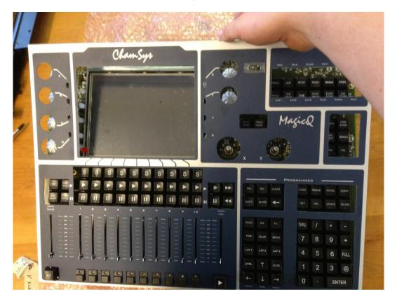
With the console at this stage, maintenance such as replacement of screen replacement, keys, encoders and faders can be carried out.
