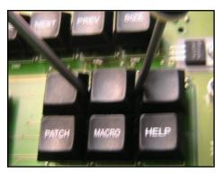
Key caps can be levered off using two flat head screwdrivers. Place one each side and apply even pressure to the key to prevent the switch from breaking. The new key cap can simply be pressed on. Key caps can be purchased individually or as an entire kit for a product.
