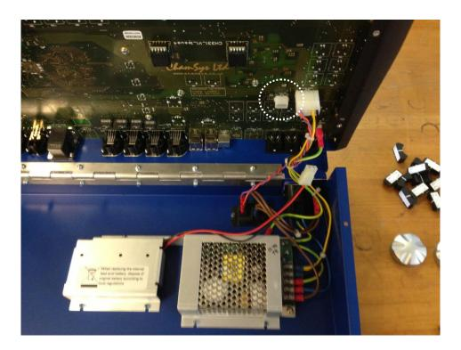
At this stage many minor repairs such as replacing the hard drive, power supply and UPS battery can be carried out, without the need to strip the console down any further.
