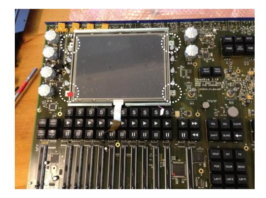
Remove the 4 M3 pozi head screws from around the edge of the screen using the 5.5mm Nut driver and Pozi 1 Screw driver.
