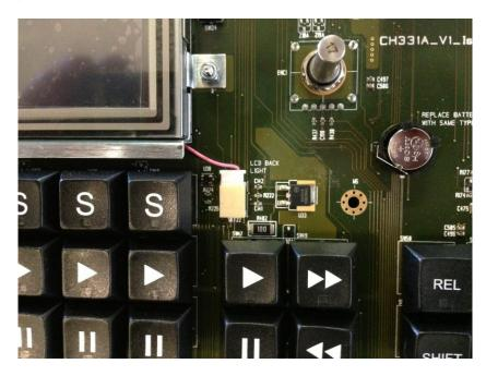
Disconnect the LCD back light connector cable located on the lower right hand side of the screen on the front panel.
