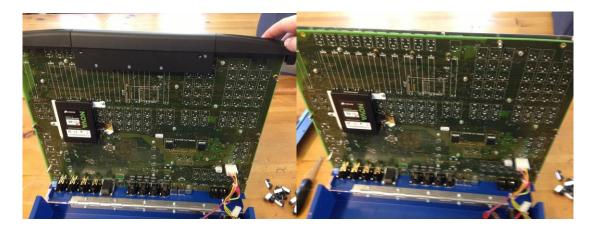
Once the side extrusions are removed the front extrusion can then be simply lifted away.
