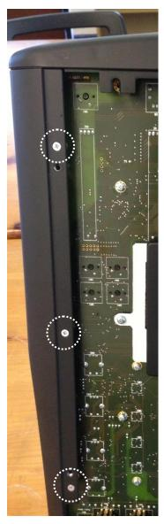
Remove the 10 of M3 x 5mm counter sunk screws on the metal extrusions.
