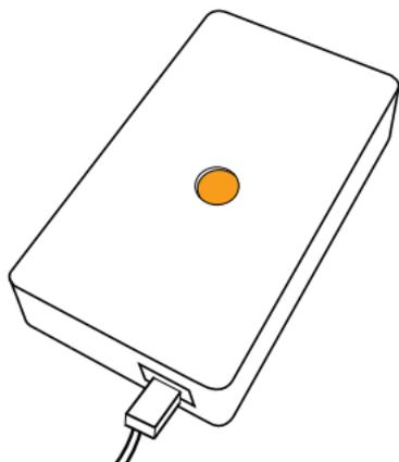
Plug Bridge into the provided power adapter and plug the power adapter into an available wall socket. You should see an LED blinking orange on the bottom side of Bridge.
