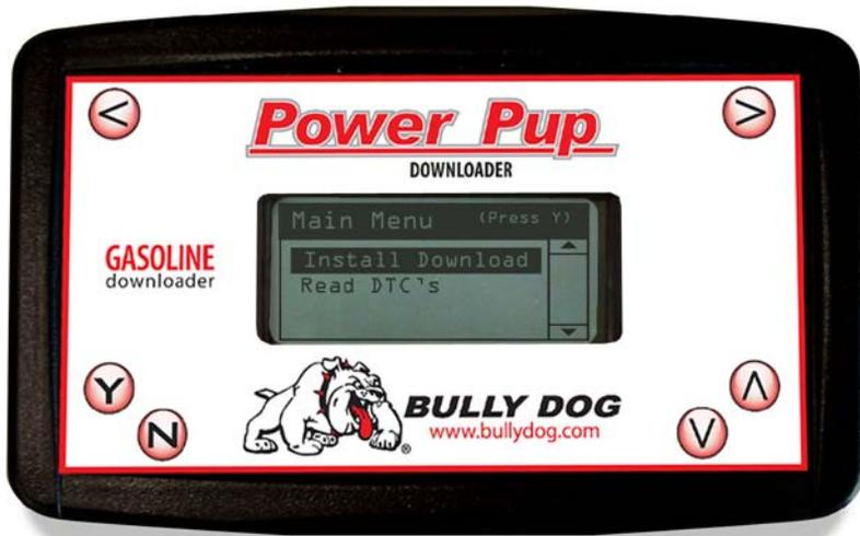
**INSTALL DOWNLOAD:** Select this option to begin the download process. Once the download process has begun it will take 15-20 minutes to complete, the process will include selecting desired power level and selecting different parameters in the vehicle specific features.
