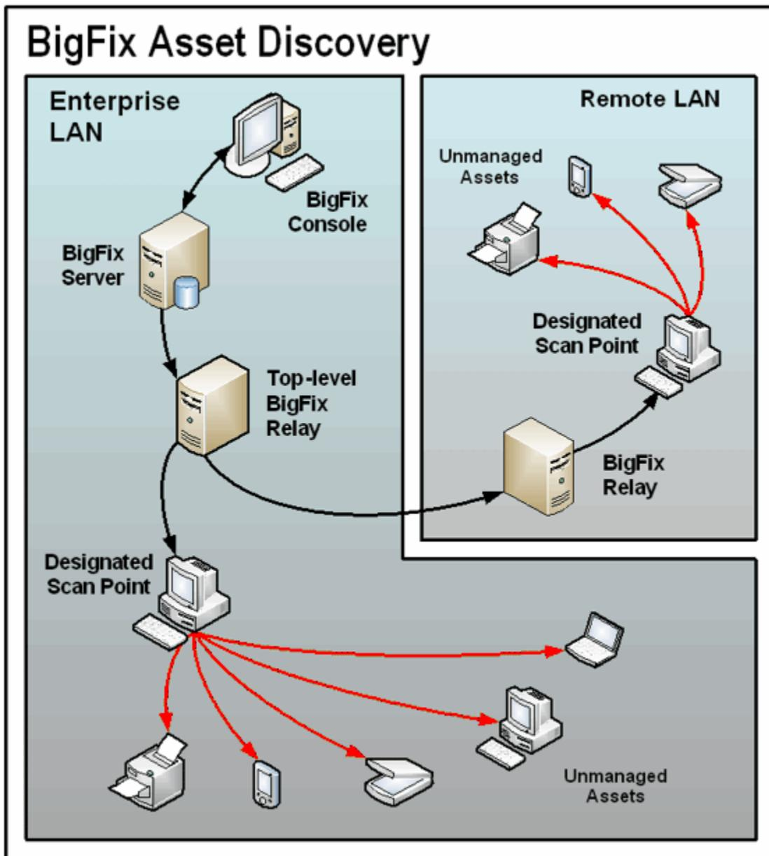
Information is retrieved from these unmanaged assets by the Scan Points and sent back through relays to the database on the BigFix server. From there, you can examine the results on the BigFix console:
