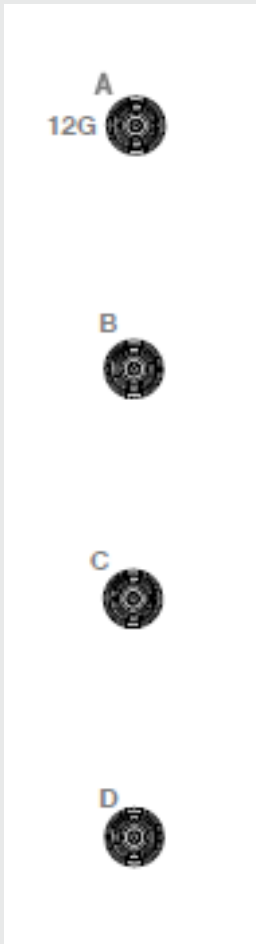
Diagram of Video Capture BNC connections on rear of unit
