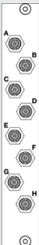
Diagram of Video Capture BNC connections on rear of a gx 2c.
