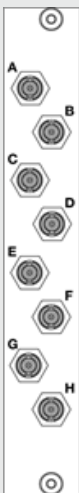
Diagram of Video Capture BNC connections on rear of a gx 2c.
